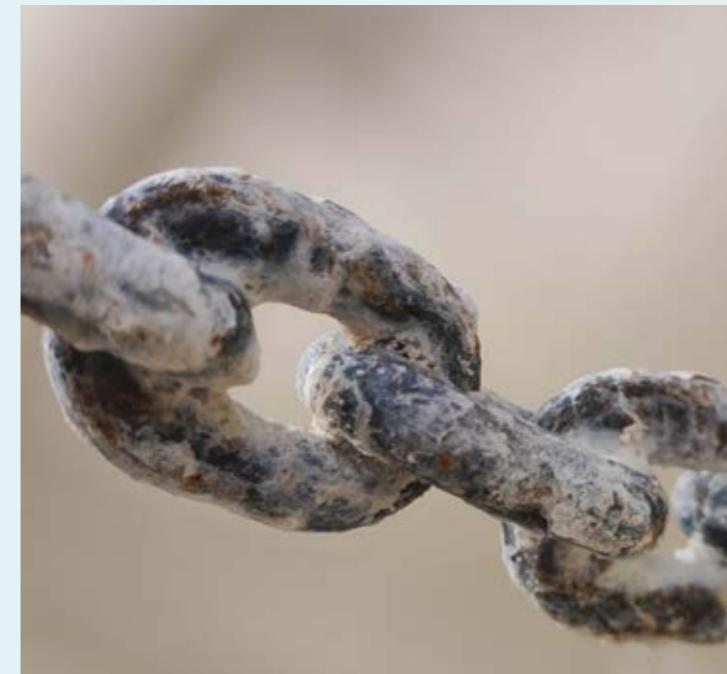
Corrosion is a process that occurs when the essential properties of a given material begin to deteriorate after exposure to recurring elements in the environment. In the case of a chain, this deterioration is evident when rust begins to appear on its links. This process, which is natural and irreversible, leads to a deterioration in the quality of the chain and a reduction in its service life.
